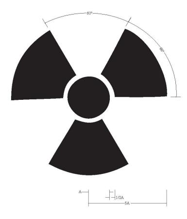
A = Radius of the central disc Note: Construction lines do not appear in the actual symbol
